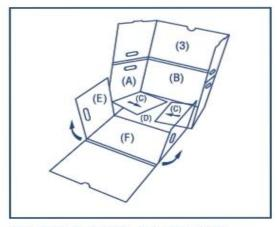
(2) STAND PANEL (B) UPRIGHT. THEN FOLD (E) UPWARD TO VERTICAL POSITION.
