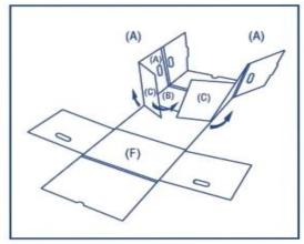
(1) FOLD PANEL (A) UPWARD THEN FOLD (C) INWARD AS SHOWN.
